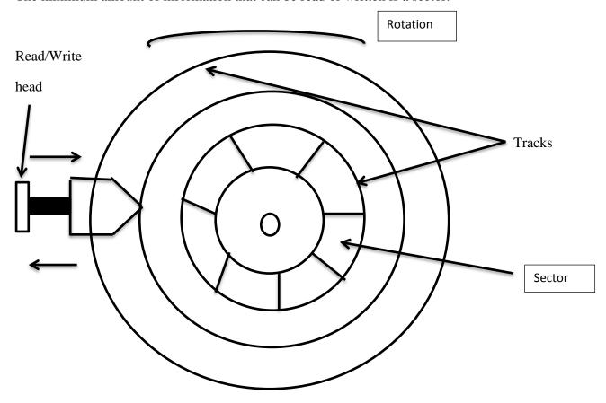
Usually several such disks may be mount on one spindle with read/write heads available on each surface. Here all disks rotate together at high speed. To read or write information to a sector it requires specifying the disk number, which surface, the sector number and the tracks within a sector.
